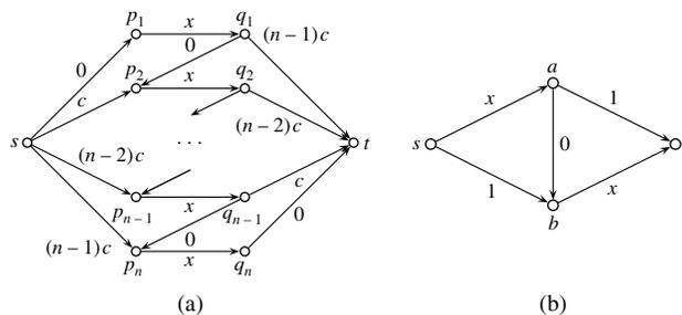
FIGURE 6. (a) Generalized Braess instance used in the proof of Theorem 6.3. (b) Braess instance. Arcs are labeled with their latency functions.
