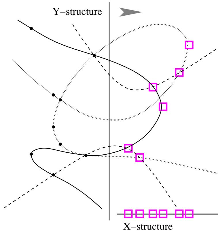
Fig. 10. Illustration of the Bentley-Ottmann sweep line algorithm.
