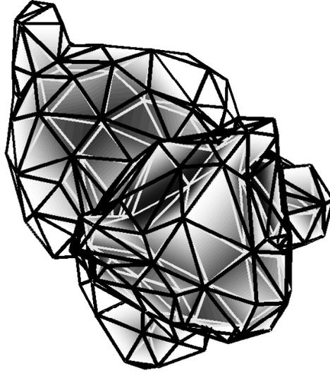
Figure 4.3: *Normal Local Compliance.* Compliance normal to the surface is shown ( $\Xi_{kk}n_k$ ). The figure is vertex colored, dark indicates a large value. Vertices not probed due to reachability constraints result in  $\Xi_{kk}^T$  not being estimated and are shown in white. A maximum of eight probes observed from two different viewpoints are employed.
