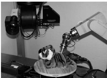
Figure 4.1: *Active Deformation Measurement in ACME: The trinocular stereocamera records the global surface deformation while the robotic probe applies a force and measures local displacement.*
