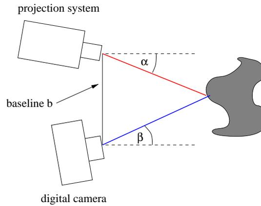
Figure 6.1: *Schematic drawing of an active stereo 3D scanner. Given the intrinsic parameters of the projection system and the camera, the baseline  $b$  and the angles  $\alpha$  and  $\beta$ , the position of a surface point can be recovered using triangulation.*
