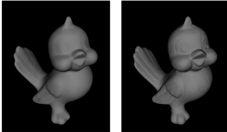
Figure 5.5: *Left: Normals of the original mesh. Right: Normals optimized using spatially varying BRDFs*
