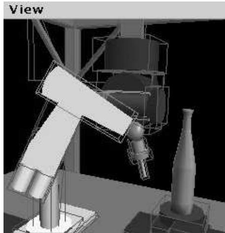
Figure 3.3: *ACME 3-D Display. A collision event produced by the simulation is rendered with the colliding boxes highlighted.*
