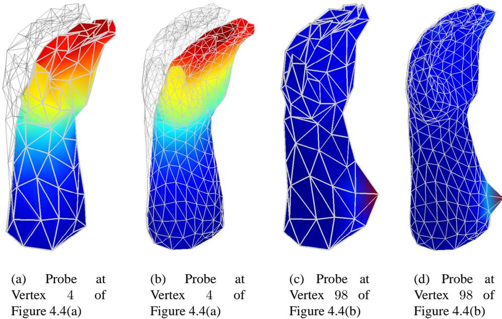
Figure 4.6: *Discrete Green’s Functions for Different Mesh Resolution. Base mesh (level 0) of the subdivision hierarchy (4.6(a) and 4.6(c)) and level 1 (4.6(b) and 4.6(d)) are shown. The estimation for both meshes is based on the same observations.*
