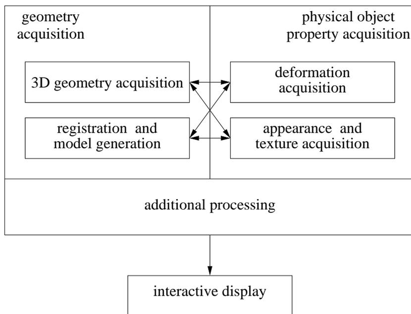
Figure 2.1: *The 3D object pipeline. Depending on the applied techniques geometry acquisition, physical object property acquisition, and registration depend on each other in different configurations.*
