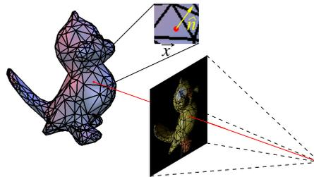
Figure 7.3: *The correspondence between pixel position and point position on the object is computed by tracing a ray through the image onto the object.*
