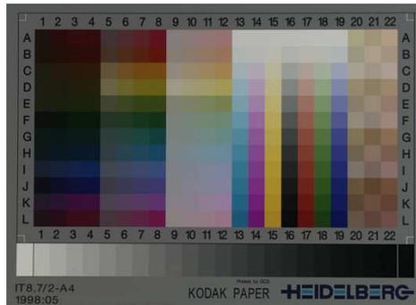
Figure 3.4: *IT8.7/2 target used to capture the color properties of an imaging system in order to generate an ICC profile.*
