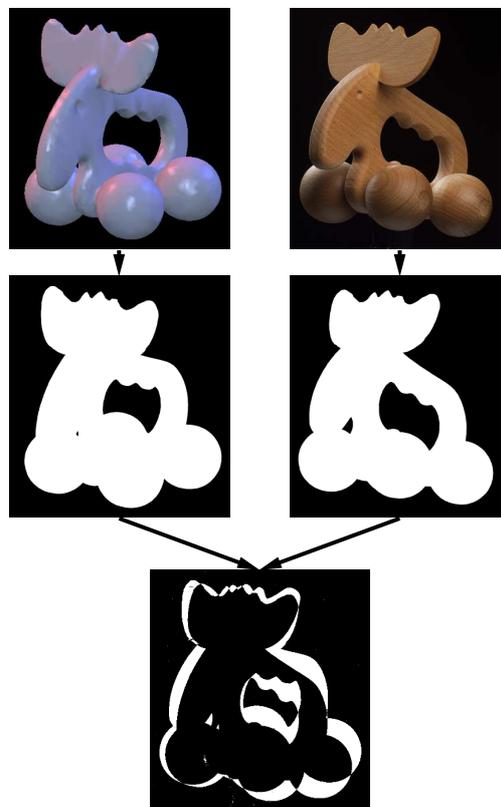
Figure 7.1: Measuring the difference between photo (right) and one view of the model (left) by the area occupied by the XOR-ed foreground pixels.
