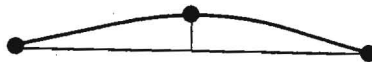
Figure 13: The curvature of an edge is measured by the distance from the supporting point in the middle of the edge to a line through the points at the ends of the edge.
