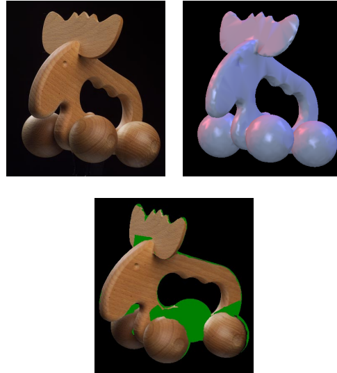
Figure 7.1: The 3D model is aligned to a captured picture which then can be mapped as a texture onto the geometry.
