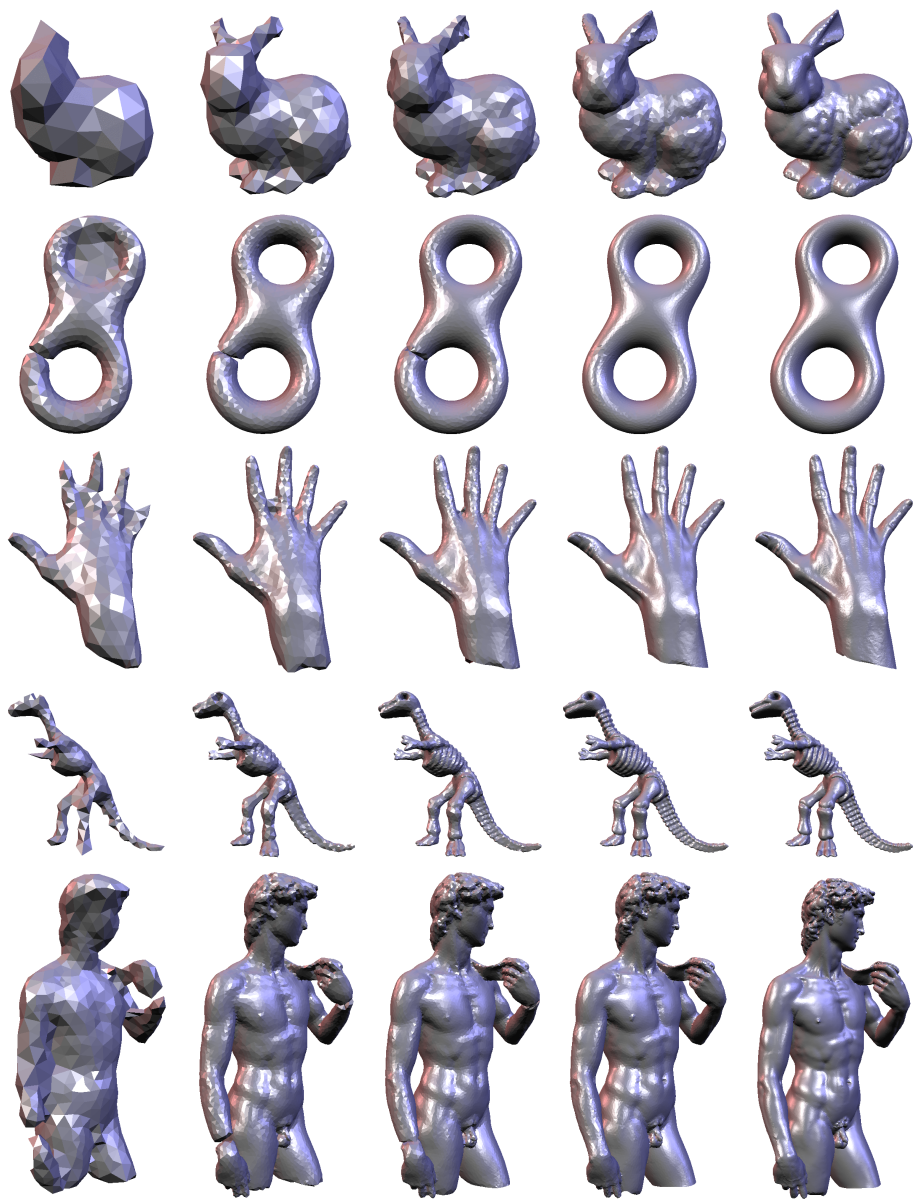
Figure 9: The Bunny, Eight, Hand, Dino and David reconstructed from 35k, 49k, 136k, 225k, 28m points, at resolution [100,500,1k,5k,20k], [1k,3k,5k,10k,15k], [500,2k,5k,20k,75k], [500,2k,5k,20k,75k], [1k,10k,17k,25k,100k], respectively.
