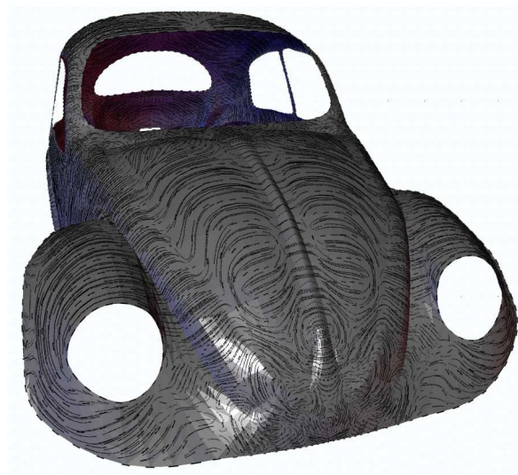
Figure 10: Lines of curvature. The (signed) maximum curvature is color coded and lines of curvature are superimposed.
