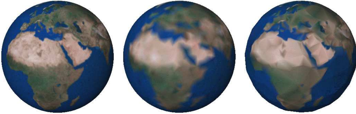
Figure 34: Example of mesh decimation using error metrics for preservation of surface attributes; left: original model (400K triangles); center: decimated without respecting color attributes (5K triangles); right: decimated preserving color discontinuities (5K triangles). The algorithm trades geometry preservation for color preservation in this case.
