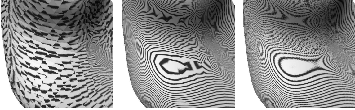
Figure 8: Reflection lines on C^0 , C^1 and C^2 surfaces. One clearly sees that the differentiability of the reflection lines is one order lower, i.e. C^{-1} , C^0 and C^1 respectively.
