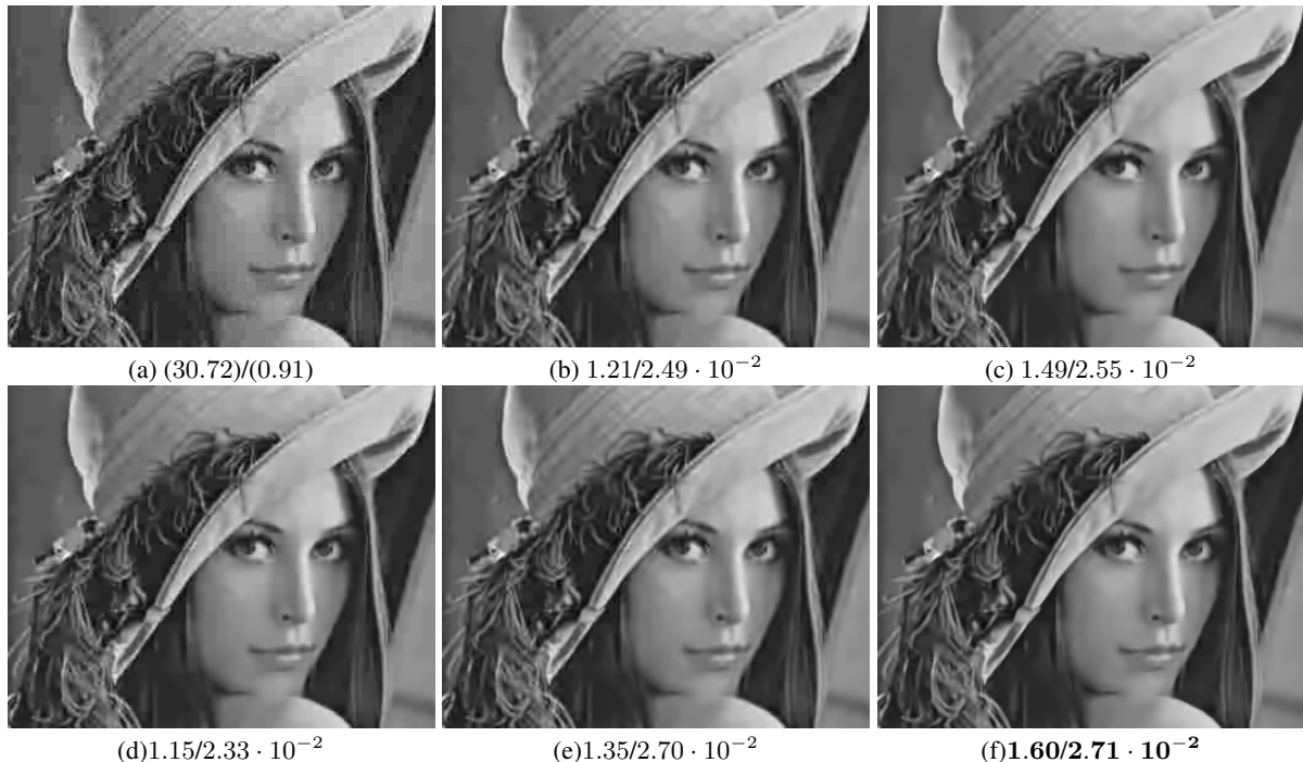
Figure 7: Examples of artifact suppression for Lena image (Q2): (a) input JPEG image, (b) re-application of JPEG [19], (c) SADCT [43], (d) FOE [3], (e) PoEdges [1], (f) our method. Increases of PSNRs (in dB) and SSIMs with respect to the input JPEG images (displayed below each column) were calculated based on the complete images. For the input image (a), the original PSNR and SSIM values are shown. The best results are marked with bold letters. Please refer to the electronic version of the current paper for better visualization.
