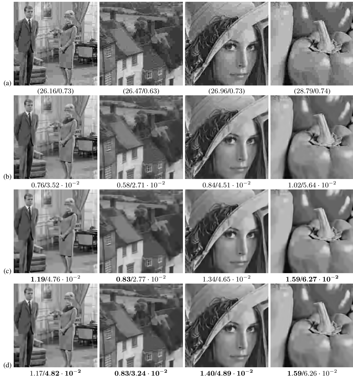
Figure 10: Examples of JPEG artifact suppression on (256 \times 256) -size sub-images (compression quality 7): (a) input JPEG images, (b) SVR-based method [23], (c) SADCT [43], and (d) our method.
