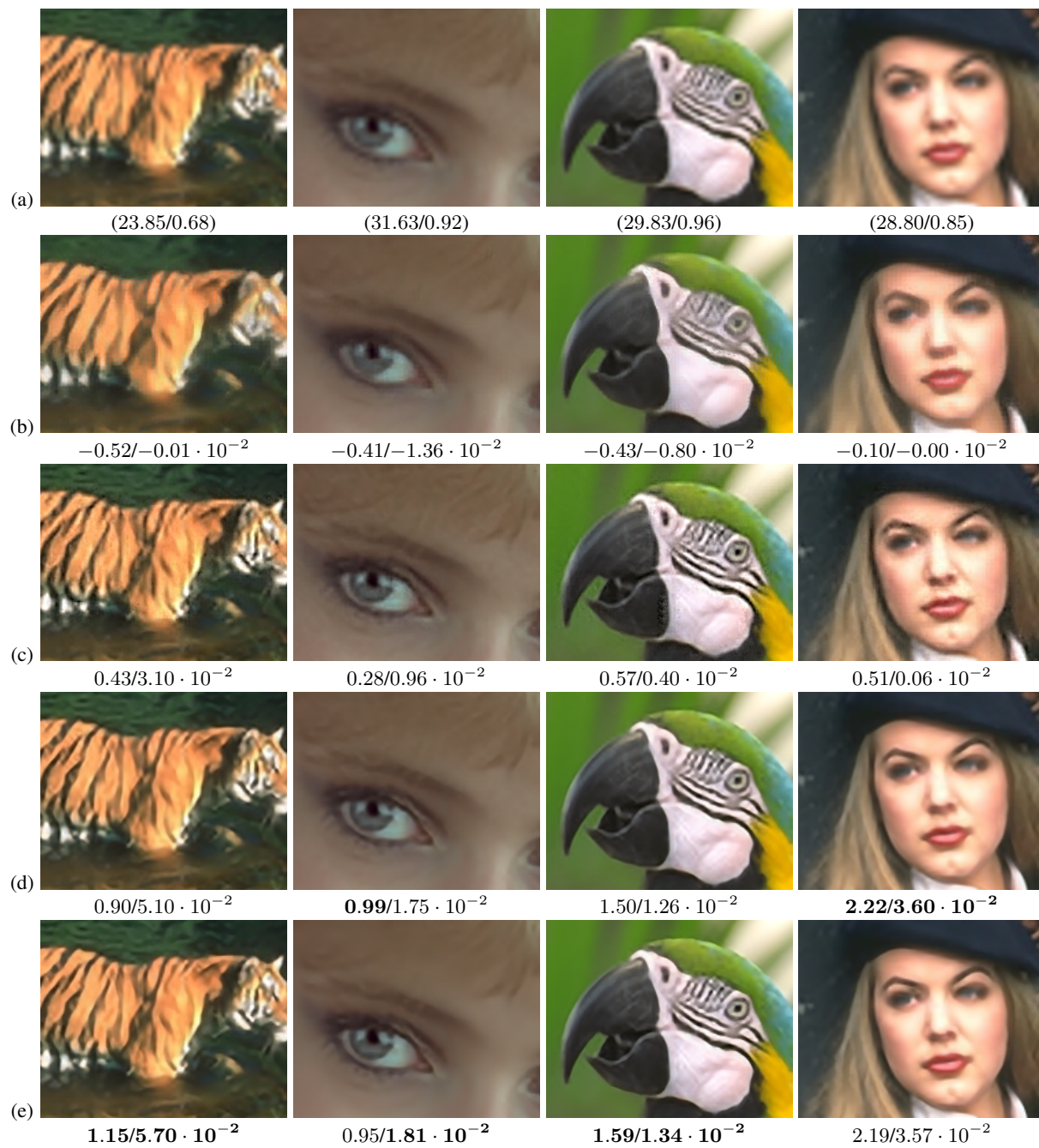
Figure 16: Examples of image super-resolution (mag. factor 3): (a) bicubic resampling, (b) Chang et al. [31], (c) Yang et al. [33], (d) Kim and Kwon [9], and (e) our method.
