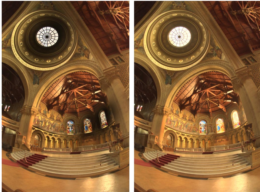
Figure 2.3: Changes made to Retinex for mapping very high contrast scenes. Dark halos around very high luminance areas (left image) were corrected by scaling world luminance to the display range (right image).
