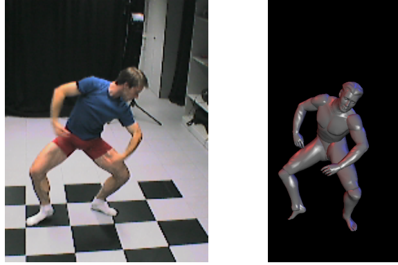
Figure 7: An input video frame (l) and the body model in the pose recovered by the motion capture algorithm (r).
