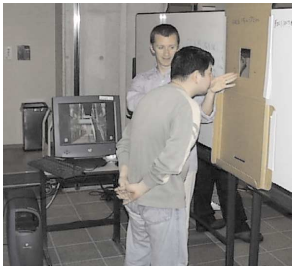
Fig. 4. Set-up used for experimental comparison of the atrium images displayed on a CRT device against the real-world view. The subject observed the atrium through an aperture which limited the field of view to the one similar to the displayed images.
