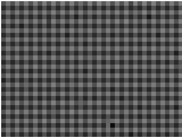
Figure 3: Excerpt of test image B taken with 25 s exposure time. Top: original version of the image. Middle: captured noise image with 25 s exposure time. Bottom: cleaned version for optimal  $k = 0.65$ . The checkerboard pattern is due to a color filter array on the CCD chip.
