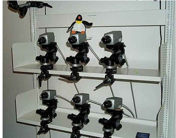
**Figure 4:** Our Lumi-Shelf, consisting of a bookshelf and six consumer-quality Fire-Wire video cameras connected to three Linux PCs.
