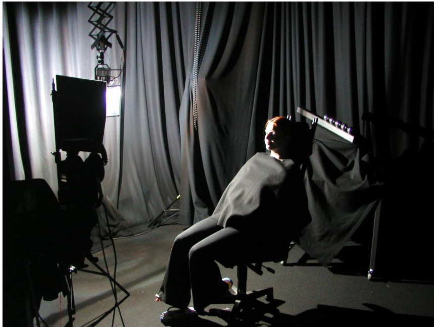
Figure 2: The measurement setup. The camera (on the left) remains at the same position, while the orientation of the subject's face and the position of the light source (which is behind a protective pane) are varied. The steel spheres behind the subject are used for measuring the position of the light source relative to the camera.
