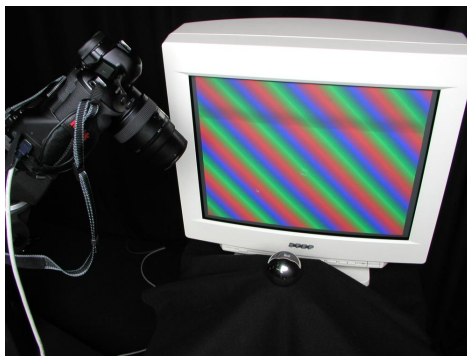
Figure 7.1: The setup used during our experiments. The patterns are displayed on a 19" CRT monitor and reflected off the target object (here the metal sphere in front of the monitor). The images are captured with a high quality digital still camera.
