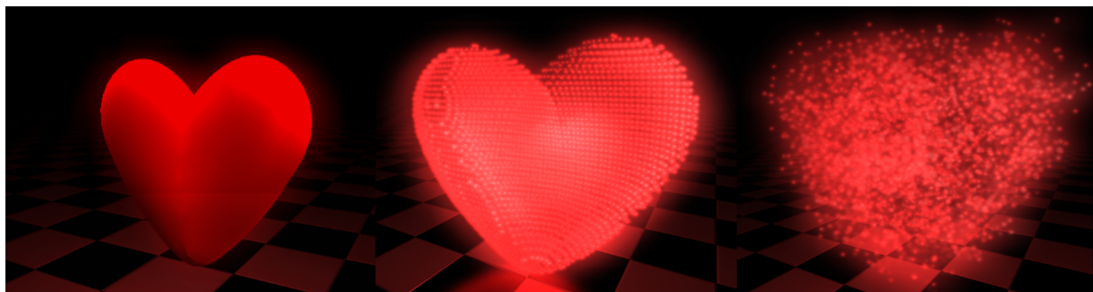
Figure 11: Screenshots from our FX demo HeartBreaker . From left to right: Solid model (5000 triangles); Point cloud representation (1872 points, in a 256x64x64 grid, first iteration: 90 ms, subsequently: 25 ms); Particle explosion effect.
